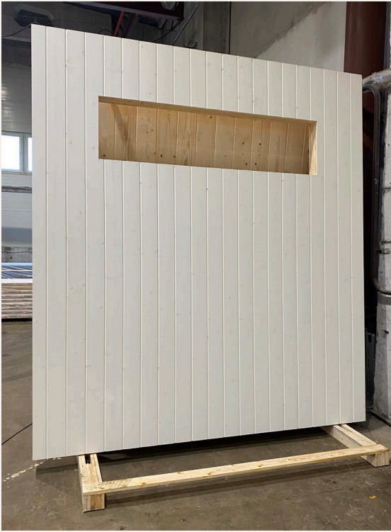
On the left image is colored visible quality panel with window cut out. On the right is colored visible quality panel with upper cut under the slope.
